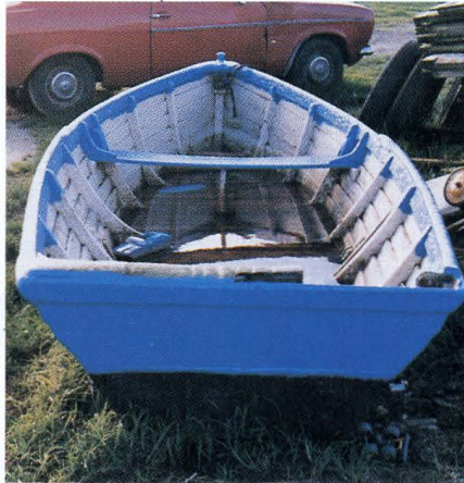
A broad-sterned Kaipara punt of a type used to carry oysters or nets aft and towed at speed by a launch. A single thwart is fitted forward. Like the Mahurangi punt, it has fore-&-aft bottom planking, clinker sides and frames sawn from natural crooks. (P. J. McCurdy)
