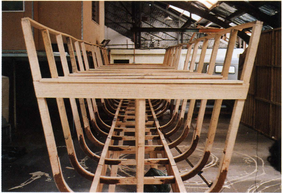
Attaching the ribs to the keels. In TE RANGIMATA sawn timber was used; in the old days they would have been of matipo.
