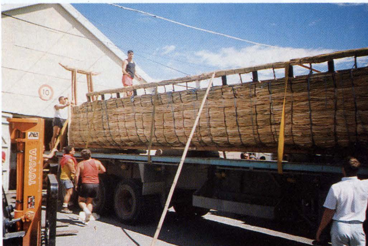
The completed waka pahi ready to be launched. The two figureheads are stylised kawau or shags; the cross-member at the stern is the small tapu mokihi.
