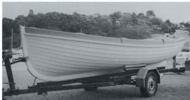
The KONTIKI, built by John Gladden of Northcote and owned by the Birkenhead Sea Scouts based at Little Shoal Bay. This view shows the straight keel, well-rounded forefoot and slightly raked stem.
