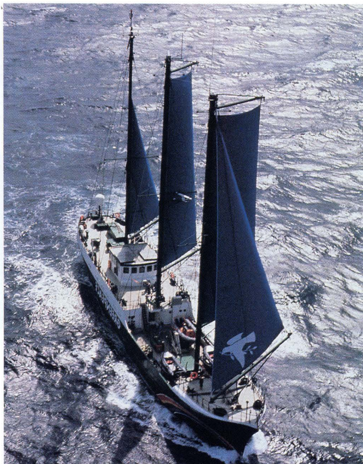
The new RAINBOW WARRIOR. The unusual three-masted schooner rig permits very fine control of sail area and trim: note the absence of twist in the gaff foresail and mainsail.
