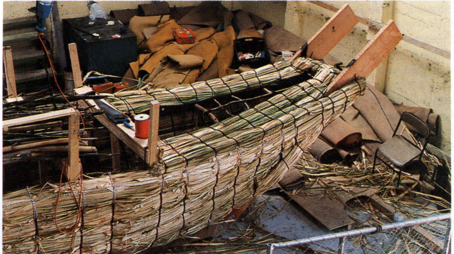
Top & Right: Pole framing and raupo decking for the foredeck.
