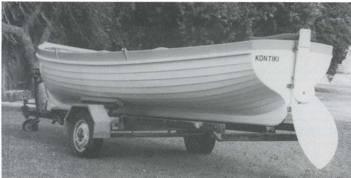
The ¾-view shows well the full bow and stern and short, rounded run. The pivoting-blade rudder is deeper than that drawn.
