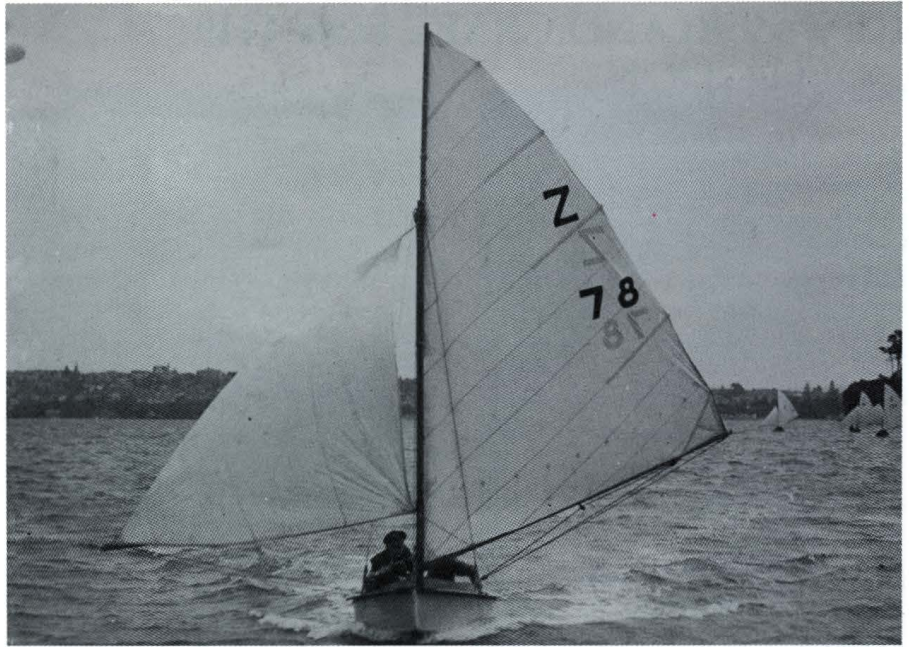
A Zeddie of the 1940s on its most exciting point of sail in a breeze. The rig comprises a gunter mainsail and a single-luff spinnaker.
