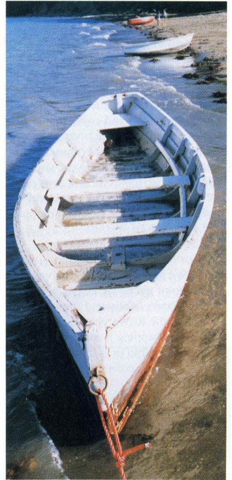
A 3-plank (per side) Mahurangi punt with a Y stern. The standard length is 22 feet and the boats were rowed and occasionally sailed. (P. J. McCurdy)
