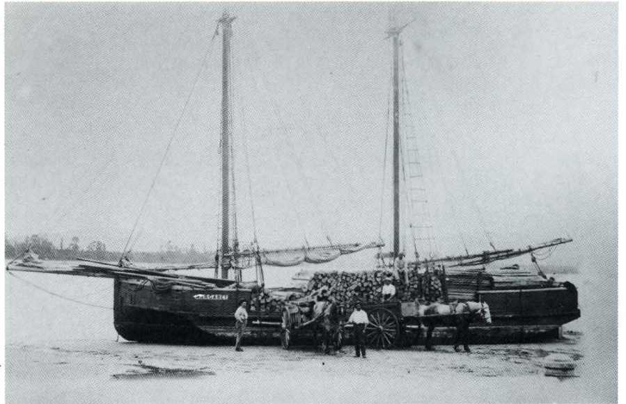
The MARGARET, with a load of split posts, sits squarely on the mud. The stem is plumb, an unusual feature in a scow. (C.W. Hawkins collection)
